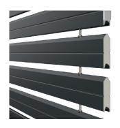
The 40-mm-high straight slats give the shutter curtain a unique elegance. They are filled with a CFC-free polyurethane foaming to improve the insulation and the stability of the shutter curtain.
