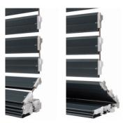
Sliding end caps made of polyamide. Excellent sliding in the side guide rails. The sliding end caps are joined together in such a way that two or three slats can be stacked together inside the storage unit at the same time. They are fixed to the slats by punching (two-slat version) or with a rustproof staple (three-slat version) and reinforced for best wind resistance.
