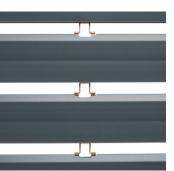
The mobile slats are joined by solid chrome-nickel steel hooks. The joining hooks can separate the slats by up to 9 mm to provide excellent ventilation and optimum lighting inside. When closed, the shutter curtain ensures complete darkness and outstanding soundproofing.
